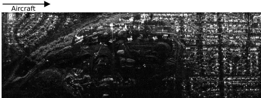
Figure 3. Stripmap SAR image of a portion of Brigham City, UT processed from data gathered using microASAR on the Surf Angel testbed. The suburban area is interrupted by a gravel pit in the center of the image which is much less reflective.
