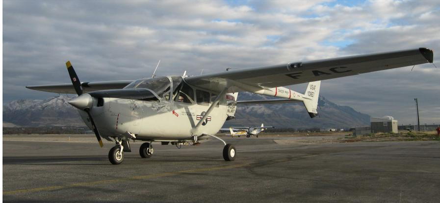
Figure 2. The O-2 Skymaster, dubbed “Surf Angel”, which is being used as an airborne SAR testbed. With the wings mounted on top of the fuselage, the pilot and radar operator can easily observe the ground below. Radar antennas are mounted beneath the aircraft and angled so that they radiate toward the passenger side.
