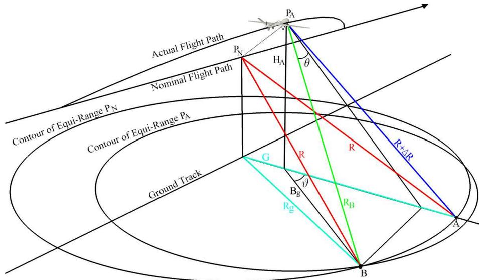
Fig. 2. The SAR platform deviates from its nominal path, point  $P_N$ , resulting in a change in range to point  $A$  from  $R$  to  $R + \Delta R$ . Point  $B$  is nominally at a range  $R$ , but the deviation to point  $P_A$  changes the range to  $R_B$ , which is different from  $\Delta R$ .
