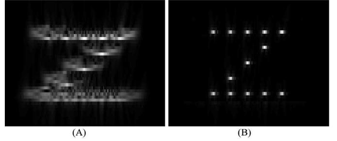
Fig. 3. Simulated LFM-CW SAR data of an array of 13 point targets with non-ideal motion (sinusoidal translational). The data is processed without motion compensation in (A) resulting in azimuth and range smearing of the targets. The same data is processed again using the motion compensation algorithms developed in this paper with the results shown in (B).
