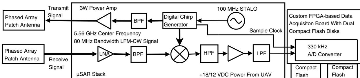
Fig. 1. Simplified BYU  $\mu$ SAR Block Diagram.
