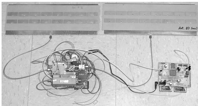
Fig. 2. Photograph of complete BYU  $\mu$ SAR system ready for flight on a small UAV.
