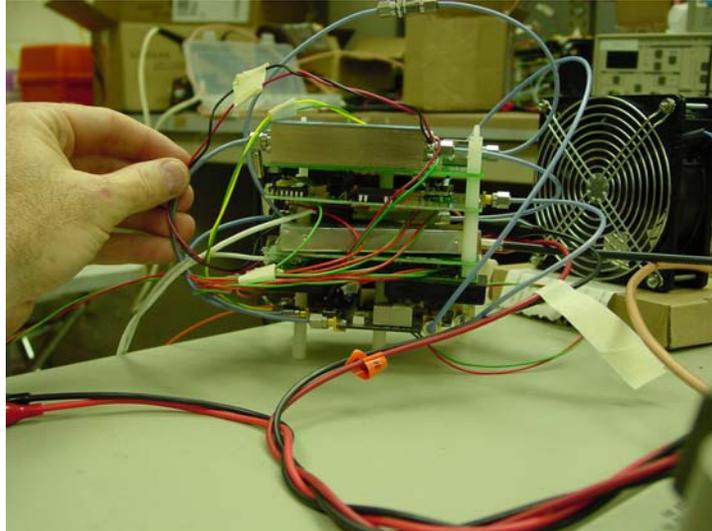
Figure 1. Photograph of microSAR RF stack. To minimize weight, no enclosure is used.
