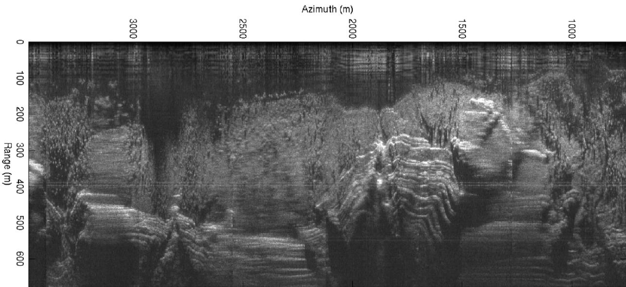
Figure 7. Example microSAR image from car-SAR driving up Provo Canyon, UT. Blurred sections result from the curving highway up the canyon. The canyon walls are naturally terraced and appear layered in the image.
