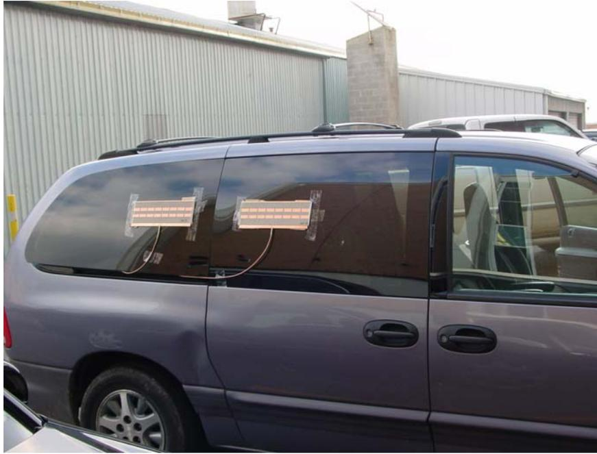
Figure 6. Testing the microSAR system on a vehicle (“car-SAR”). Note orientation of antennas relative to motion direction and the direction of the patches.
