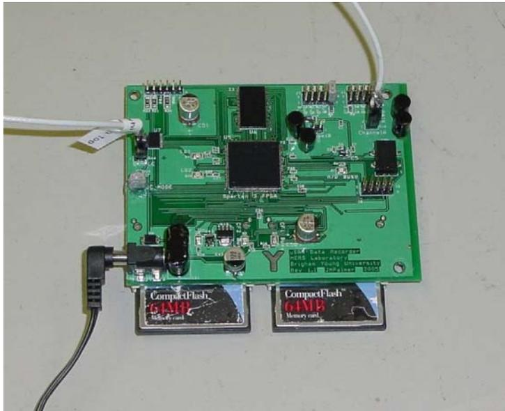
Figure 2. microSAR data acquisition module consisting of a PC104 A/D and single board computer. Data is stored on Compact Flash devices.
