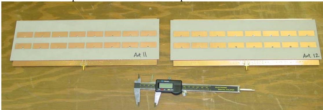
Figure 3. microSAR antennas consisting of two flat panels made out of high frequency circuit board material. Each is connected to the RF stack using a single RF cable. They are mounted with the long direction aligned with the flight direction with the radiating side (shown) pointed to one side of the vehicle.
