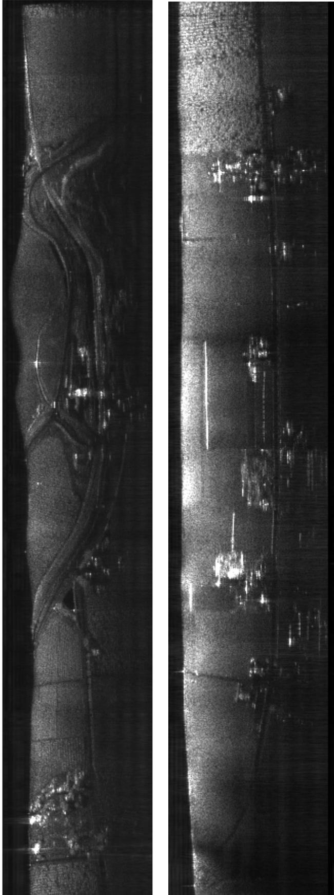
Figure 8. Example microSAR images collected from a small manned aircraft near Benjamin, UT.
