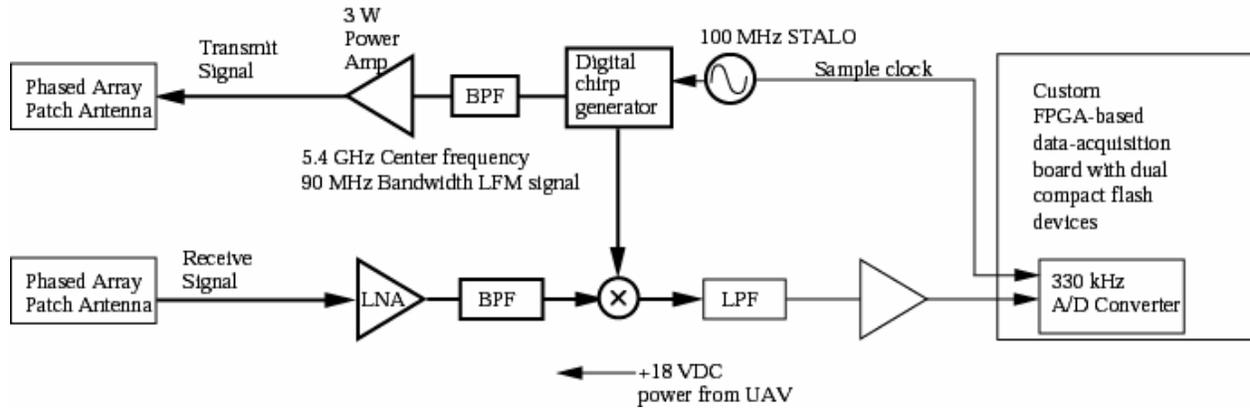
Figure 4. BYU microSAR block diagram.
