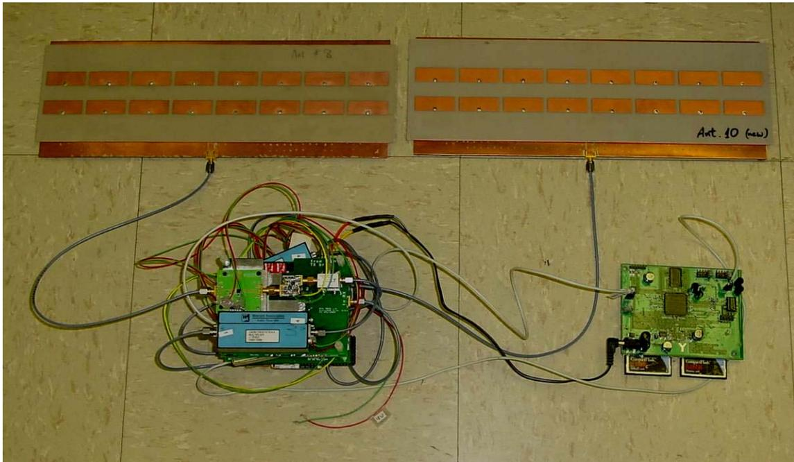
Figure 5. Photograph of complete BYU microSAR system ready for flight on a small UAV.
